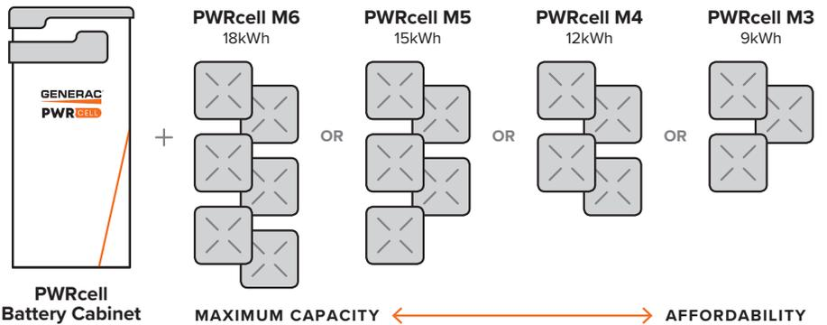
While some manufacturers only offer a one-size-fits-all system, PWRcell can grow with your household as your energy needs increase. The standard PWRcell system includes three battery modules that offer 9 kilowatt-hours (kWh) of storage capacity. It can expand in increments of 3kWh up to 36kWh using a single inverter.
